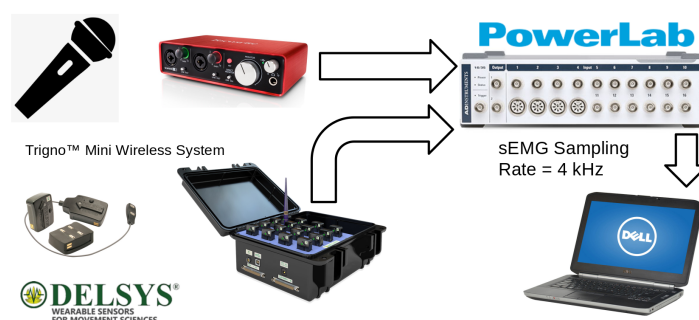
Figure 1. System setup for data collection showing the flow of signals through the equipment.
